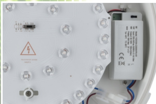
Easily accessible CCT & Power changeable switches
