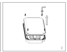
Use the provided Allen key to unscrew the 4 diffuser screws and remove the diffuser
