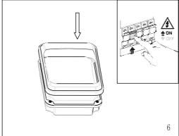
Clip the cover back onto the fitting and turn on mains supply to test the wall pack.
