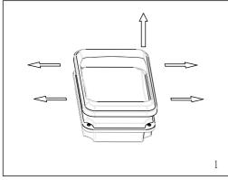
Unclip the cover to access the diffuser screws.
