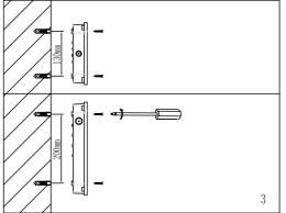
Fix the base to the wall using adequate fixings, ensuring the fixing surface is even and flat.
