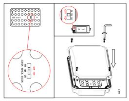
Select the CCT from the switch on the LED board and the power required from the switch located on the driver and screw back the diffuser making sure the base seal is in place and undamaged.
