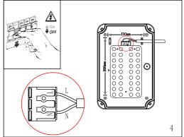
Use any side for cable entry, create a 20mm hole to fit the included gland. Pass the wires through the gland and connect them as per the wiring above.
