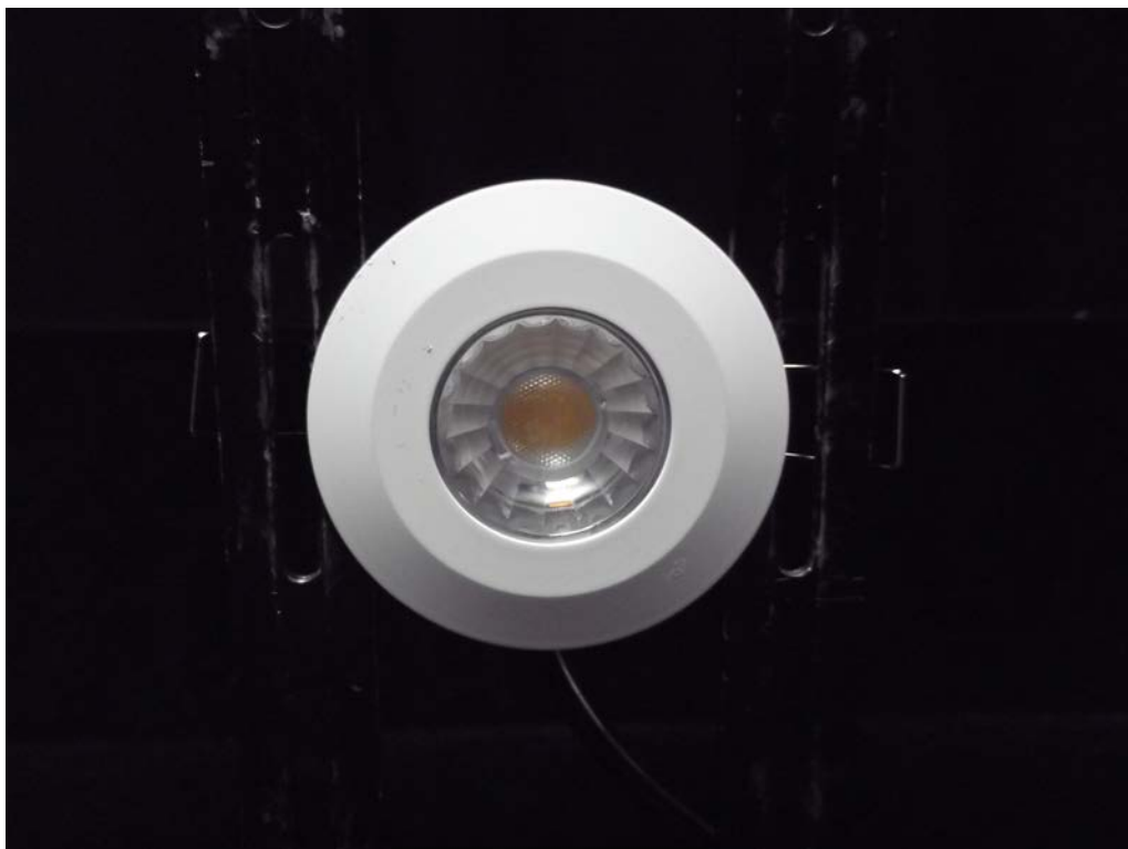
Photo 1: Luminaire on goniometer mount
