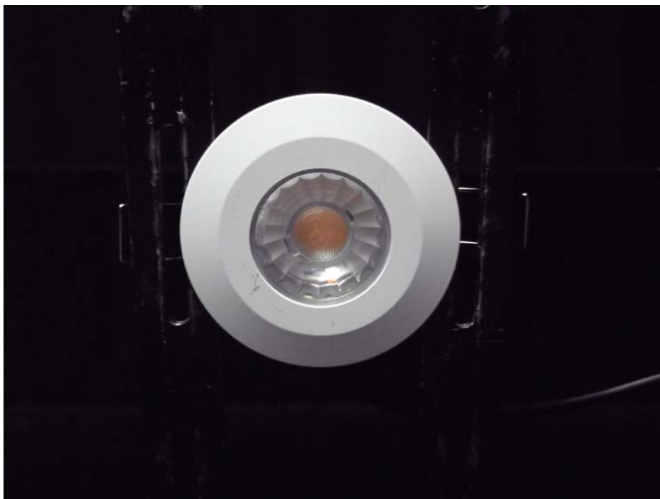
Photo 1: Luminaire on goniometer mount
