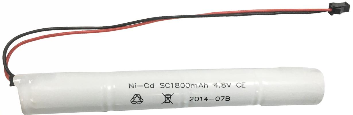
This is a sealed 4.8 volt, nickel cadmium rechargeable 4 cell battery stick complete with amp plug for use with LTDL3NM 3W emergency downlight.
