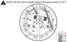
Open the LED gear tray and use the driver DIP switch to change the power
