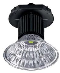
New Flip Chip High Bay is a perfect combination of packaging and thermal management. The ceramic-based flip chip LED is reflow-soldered directly to the MGCP heat sink resulting in super fast heat transfer with more than 3 thermal resistance layers reduced.
