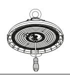
2. Install the sensor on the sensor base and tighten it.
