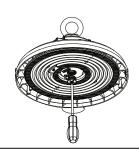
2. Install the sensor on the sensor base and tighten it.
