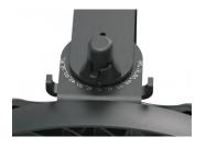
Adjustable Beam Angle: Our unique adjustable bracket wall / ceiling / pole bracket gives you greater beam angles up to  $\pm -90^{\circ}$ . It requires no tools to fix the high bay angle and is secured with a high quality spring loaded bolt assembly which keeps the unit locked in the correct position even in outdoor conditions.
