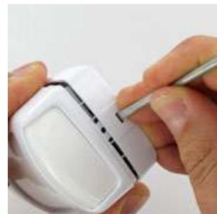
3. Hold the battery in place, and then pull out the battery tab to power up the sensor.
