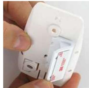
2. Open the sensor using the tool provided.
