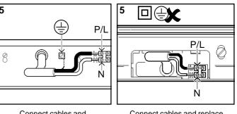
Connect cables and replace lamp and diffuser.
