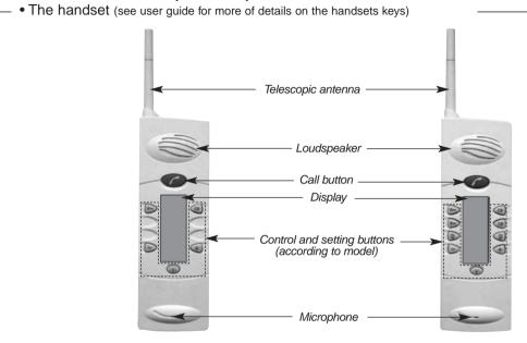
NB: the battery cover is located at the rear of the handset
