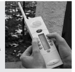
NB: if there has been neither a beep nor a display, radio recognition has failed. Start the procedure again from the beginning ensuring you leave at least 3 seconds between pressing the button on the controller and the button on the external caller unit, and that you keep the handset at least 2m from the controller.
