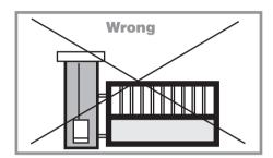
• never run a cable along the antenna (particularly the link cable between the external caller unit and the controller),
