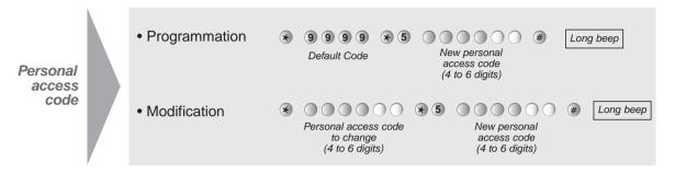
Please note: during programming, all programming errors (erroneous access code, incorrect number press, too brief press...), are signalled by three short BEEPs or by one warning BEEP!
