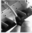
**Ensure correct orientation** of the grommets.
