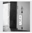
The indoor station must be fixed to the wall. Locate a flat surface. For ease of use, we advise you to mount the indoor station at about 1.5m high.
