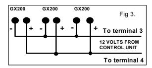
Each detector requires 12 volts DC in order to operate and this is connected to the + and - terminals. The 12 volts must be wired in "PARALLEL" as shown in (fig.3).
