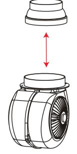
Reducer Collar reduces the motor exhaust from 150mm to 125mm if required (Already supplied in box)
