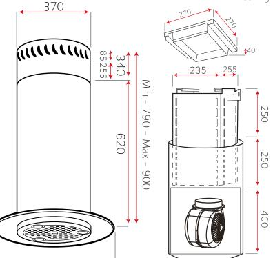
Please note the Subframe for the LA-RND Isl is adjustable and has a sliding mechanism on the ceiling bracket for easy installation.
