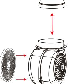
Reducer Collar reduces the motor exhaust from 150mm to 125mm if required (Already supplied in box)
