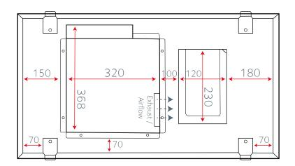
Ducting - Our slimline motor is designed with a rectangular ducting system. Please note as this ducting is rectangular and not round, it will have different dimensions.
