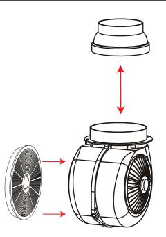
Reducer Collar reduces the motor exhaust from 150mm to 125mm if required (Already supplied in box)
