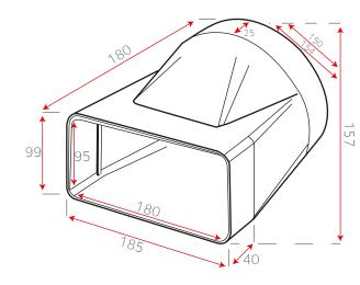
Ducting – Our slimline motor is designed with a rectangular ducting system. Please note as this ducting is rectangular and not round, it will have different dimensions.
