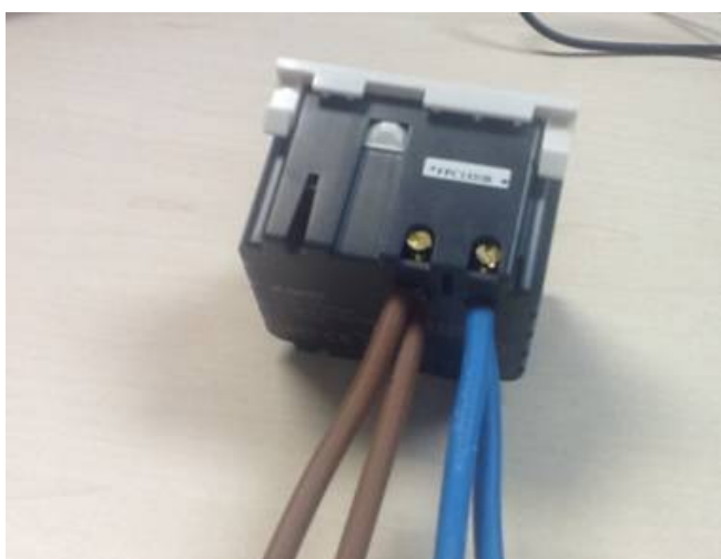
Fig 2 - K5837WHI USB Charging module - top view with 2x 4mm 2 cables
