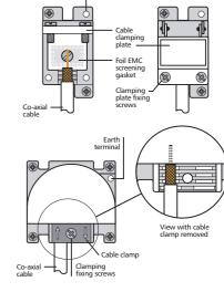
In the event that the earth terminal is required to be used, the installer must ensure that a suitable earth conductor is present to connect to the earth terminal. (In the case of 2G products both TV modules should be earthed).
