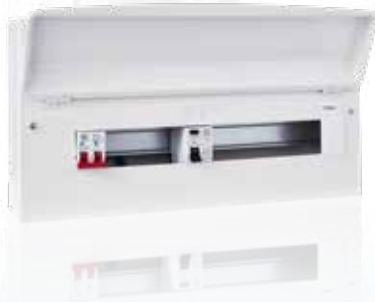
Y5684sMET 21 WAY ENCLOSURE 100A SWITCH DISCONNECTOR 80A 30MA RCD ACCEPTS A FURTHER 17 ONE MODULE PRODUCTS
