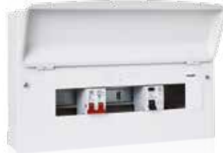
Y5685sMET 16 WAY ENCLOSURE 100A SWITCH DISCONNECTOR 80A 30MA RCD ACCEPTS A FURTHER 12 ONE MODULE PRODUCTS
