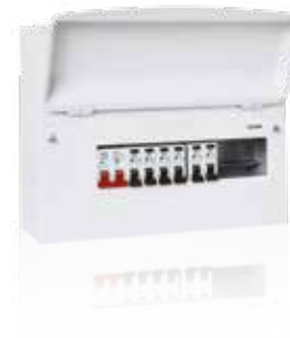
Y7673sMET 12 WAY ENCLOSURE 100A SWITCH DISCONNECTOR 6 X RCBOs (2 X 6A, 1 X 16A, 2 X 32A AND 1 X 40A) ACCEPTS A FURTHER 4 ONE MODULE PRODUCTS
