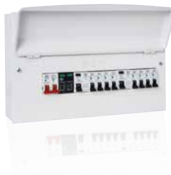
YS8666sMET 16 WAY ENCLOSURE 2 X 100A 30MA RCD 8 X MCBS (2 X 6A, 2 X 16A, 3 X 32A, 1 X 40A) 1 X SURGE
