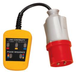
For 3-phase socket outlets, the PC101 will instantly prove connection of all three lines (or identify which are not connected) and show the sequence of phase rotation. Essential to ensure correct and safe running of three phase plant, it is fitted with a red 16A, 3P+E BS4343/ IEC309 plug.
