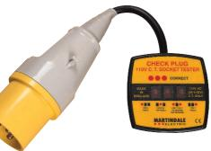
Using LED's to highlight possible fault combinations, the CP301 is invaluable for instantly checking sockets in a factory or on site installations.
