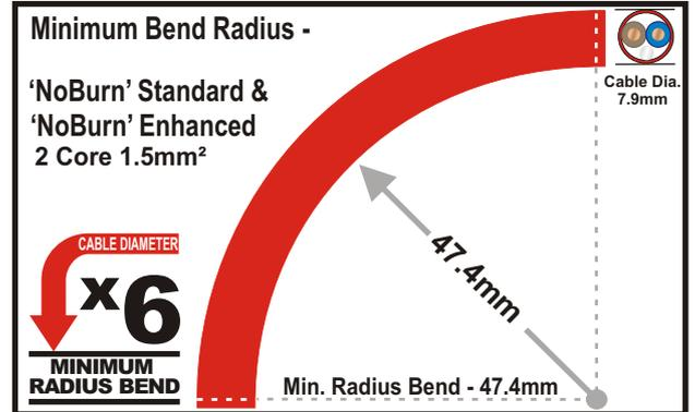
For NoBurn Platinum 'Standard' and NoBurn Diamond 'Enhanced' cable we recommend a minimum bend radius of 6 x diameter.
