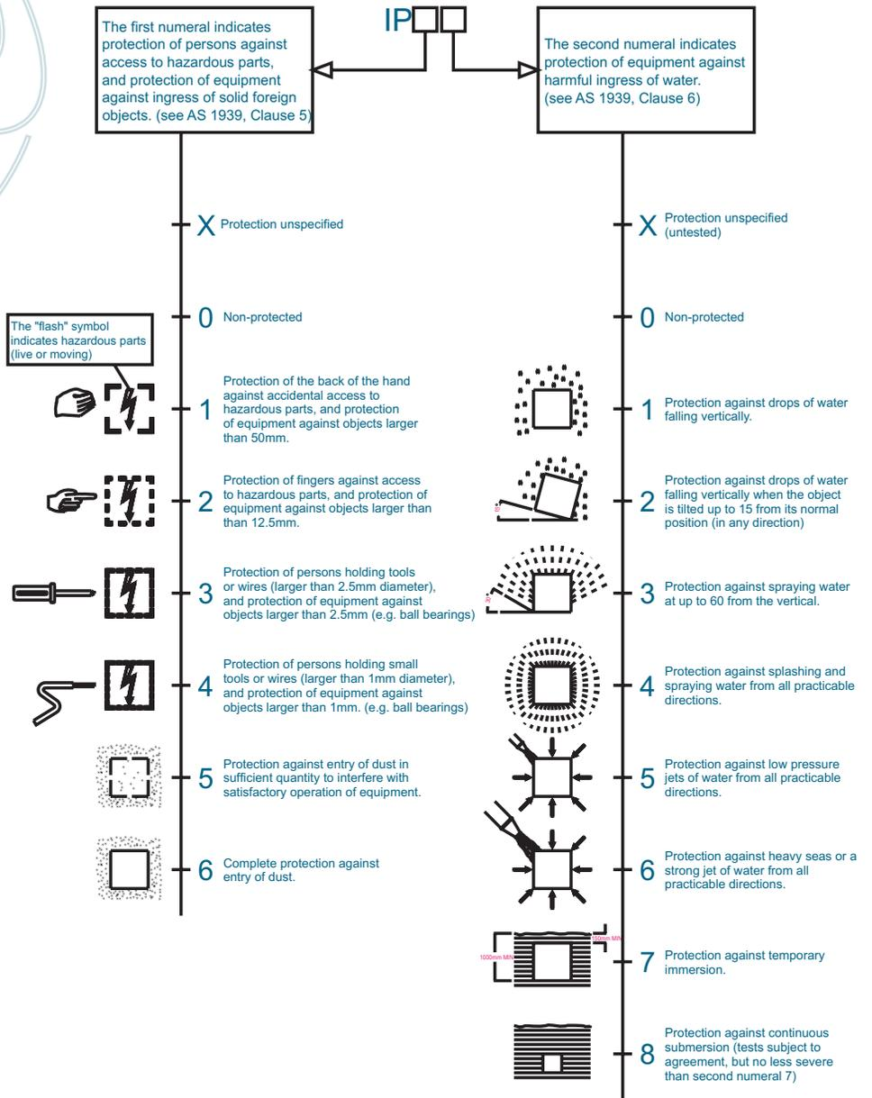
The IP 68 degree of protection is a characteristic of boxes and enclosures, but we are unable to label the Gel joints as IP 68 but instead we have to label them **IP X8**.
