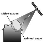
Although they are not included in this kit, a compass and a satellite finder meter are very useful tools to help you locate the satellite and set your dish in the optimum position.
