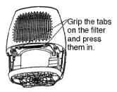
To clean the filter, first remove the bucket, the tab of the filter will then be visible behind the front grille.
