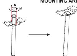
To assemble the mounting arm slide the mounting plate (L) over the collar post and fit the mounting cap (M). Secure the cap to the plate using 2 x M5 screws (N). This allows the post to rotate even after fixing.
