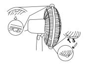
Attach the front grille (1) to the rear grille (7) using the grille clamp (3), and tighten the fixing screw (2) to retain in place.
