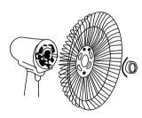
Rotate the grille fixing nut (6) anticlockwise to remove it from the motor housing. Locate the rear grille (7) on to the motor housing (10) and fix in place with the grille fixing nut (6).
