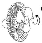
Place the blades (5) on the motor shaft (8), and locate the peg (9) into the recess at the back of the blades. Fix the blades in place using the blade fixing nut (4). Rotate anticlockwise to tighten (it has a left-handed thread)
