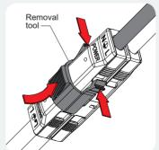
Mount removal tool. Place thumb on thumb grip and using other hand, squeeze side arms so they locate beneath the snaps.
