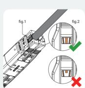
Check there is a sufficient length of outer cable sheath available for clamping. (fig.1) and that an unbroken length of conductor occupies the full extent of the window (fig.2).
