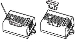
Replacing the fuse
