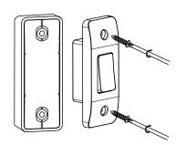
Note - The QUASW Architrave Wireless Switch is compatible with 1 Gang Architrave flush or surface boxes with 16mm minimum depth.
