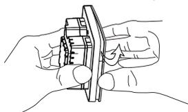
Fig.3 Carefully open the switch panel
