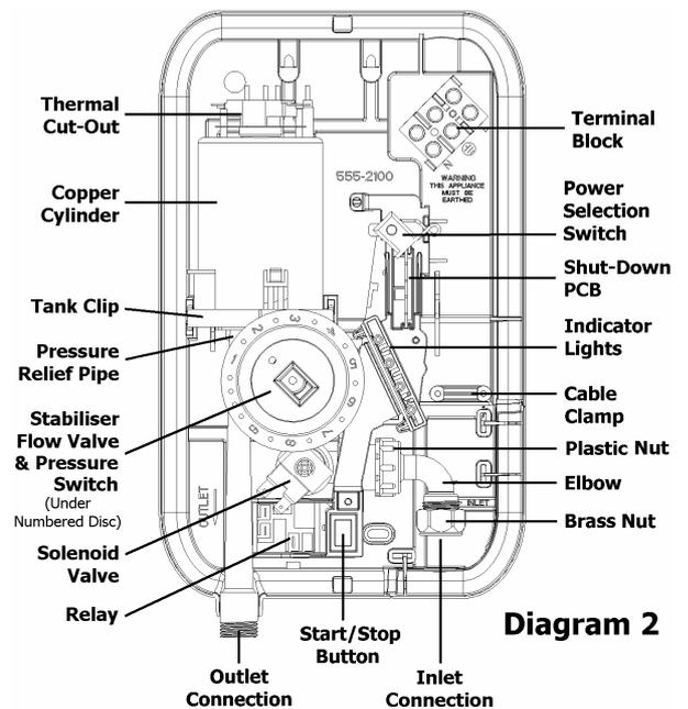
5. If the water supply falls below a set limit, the pressure switch will operate and switch off the power to the elements. This is indicated by the middle power indication lights flickering and going out (see "Effect of Other Water Devices on Incoming Water Supply").
