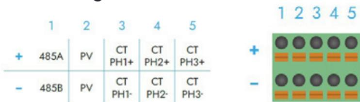
The connected EV Chargers need to have balancer multi-charger management enabled. Connect to each charger via the BG SyncEV Charger Set up App.
