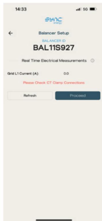
**Please Note:** A minimum of 3 amps is required to ensure correct CT connection, Press Refresh to retrieve the latest readings.
