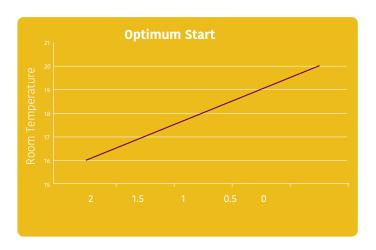
The 2-hour optimisation period and the 2°C per hour assumed temperature rise are non-adjustable. The optimisation process will be cancelled if any overrides are used during the 2-hour period of operation.
