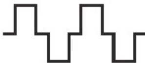
MODIFIED SINE WAVE (MSW)
