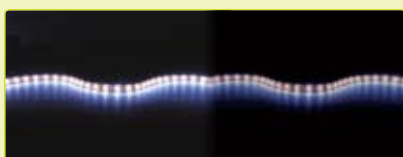
Bright LEDs 10cm from power source Dim LEDs 20.0m from power source
