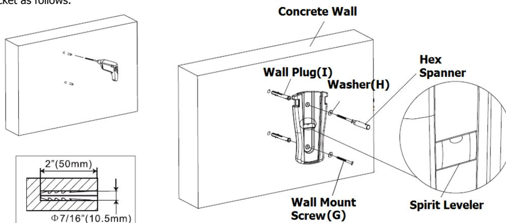
For plaster wall installation first of all find out where the wood stud is behind the wall using a stud finder. Then work out the height of the installation and ensure it is level using the spirit level. Use a pencil to mark where the mounting holes will be and use an electric drill to drill a hole that is around 4.5mm in diameter and 50mm deep. Install the wall bracket as follows.
