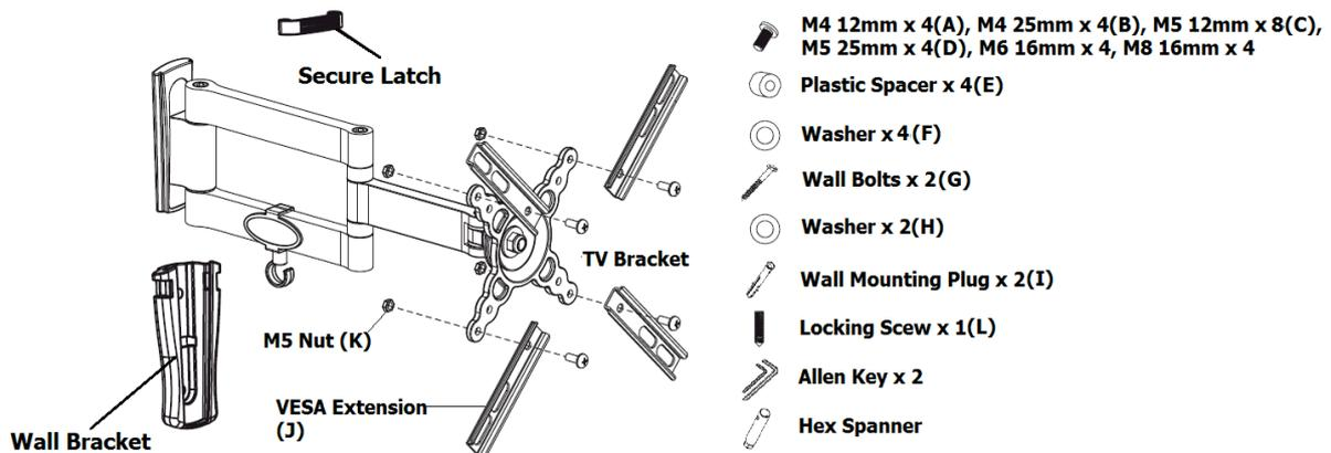
For this installation you will also require a pencil, tape measurer, electric drill, stud finder and a Philips (cross) screw driver.
