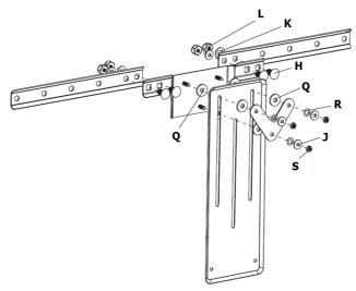
Step 2 – Attach the long part of the soundbar bracket to the adaptor as shown below.
