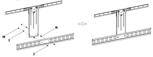
**Step 3** – Check the back of the soundbar and identify the best mounting points. Install the soundbar bracket accordingly by 4, 2 or 1 screws per side. Does not require washer if M6(G) is used for mounting.
