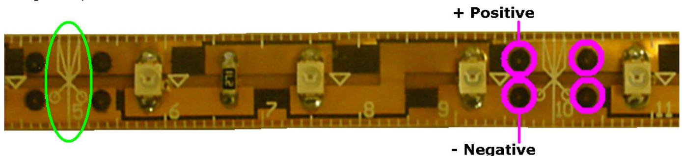
At either side of the cutting points are the DC connectors. If you want to extend these a DC cable can be soldered to them in order to connect more tape.
