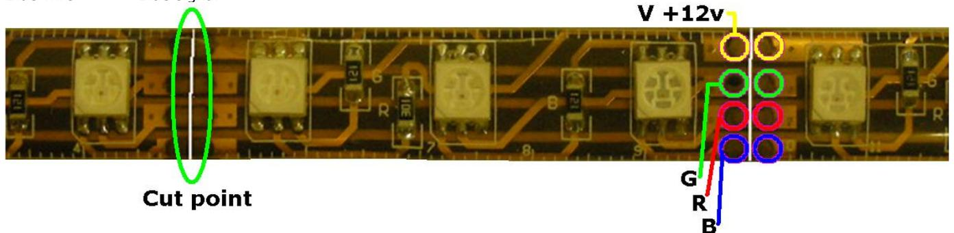
Each individual LED on the tape has three colour diodes mounted inside. They are the primary colours of Red, Green and Blue. When set at different intensities the light mixes and can produce many different colours
