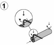
Push the L-shaped hexagon key provided fully down into the black plastic screw heads on the side of the tube at each end. To release the outer tube you must tighten both screws inwards by rotating the screw heads **clockwise**. Push one end of the plastic inner cylinder and slide the tube off, revealing three sections joined together. Pull these sections apart so that you are left with the outer tube and three sections of the plastic inner cylinder.
