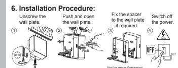
Fix the spacer with the wall plate to the wall or the wall plate alone.
