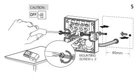
5.7 Terminate the 230V 50Hz mains supply cable into the terminal block (See image 6) ensuring correct polarity is observed and that all bare conductors are sleeved (See section 6. Connection Diagram – for wiring details).
