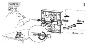
4.7 Terminate the 230V 50Hz mains supply cable into the terminal block (See image 6) ensuring correct polarity is observed and that all bare conductors are sleeved (See section 5. Connection Diagram – for wiring details).
