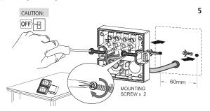
5.7 Terminate the 230V 50Hz mains supply cable into the terminal block (See image 6) ensuring correct polarity is observed and that all bare conductors are sleeved (See section 6. Connection Diagram – for wiring details).
