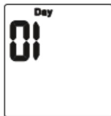
Use the Adv/Ovr or boost button to adjust the hour to the correct hour. Press Time to set the hour, and then the time will show the minutes. The hour is a 24 hour clock.
