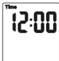
Use the Adv/Ovr or boost button to adjust the minutes to the correct minutes.
